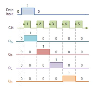
Note that after the fourth clock pulse has ended the 4-bits of data (0-0-0-1) are stored in the register and will remain there provided clocking of the register has stopped. In practice the input data to the register may consist of various combinations of logic "1" and "0". Commonly available SIPOIC's include the standard 8-bit 74LS164 or the 74LS594.
