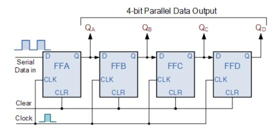
The operation is as follows. Lets assume that all the flip-flops (FFA to FFD) have just been RESET (CLEAR input) and that all the outputs  $Q_A$  to  $Q_D$  are at logic level "0" ie, no parallel data output.
