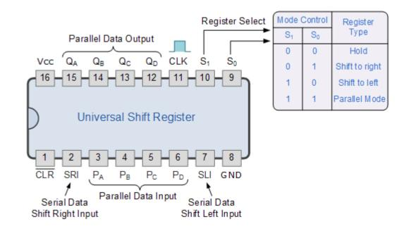
Universal shift registers are very useful digital devices. They can be configured to respond to operations that require some form of temporary memory storage or for the delay of information such as the SISO or PIPO configuration modes or transfer data from one point to another in either a serial or parallel format. Universal shift registers are frequently used in arithmetic operations to shift data to the left or right for multiplication or division.
