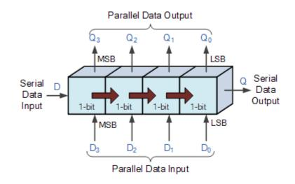
Also, the directional movement of the data through a shift register can be either to the left, (left shifting) to the right, (right shifting) left-in but right-out, (rotation) or both left and right shifting within the same register thereby making it *bidirectional*. In this tutorial it is assumed that all the data shifts to the right, (right shifting).
