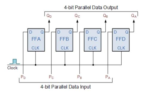
The PIPO shift register is the simplest of the four configurations as it has only three connections, the parallel input (PI) which determines what enters the flip-flop, the parallel output (PO) and the sequencing clock signal (Clk).
